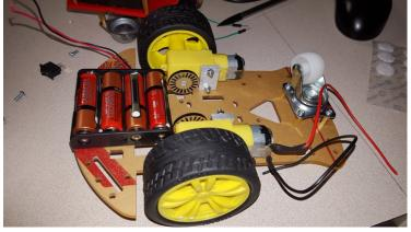
Hint- battery pack has to be attached someplace that it does not "tip" the robot.
